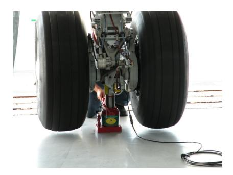
If the jacks run out of lift prior to clearing the ground then jack adapters should have been used. In some conditions,  $\frac{1}{2}$  inch shim plates can be placed under the tires and or jacks to shim accordingly to obtain the proper lift.
