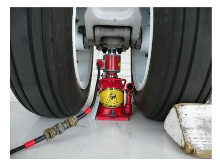
If more than one inch clearance an over the top jack adapter will be required as shown below:
