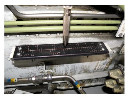
With jacks in place and load cells connected, check that there is no contact with the cells to the jack points. Check the zero of the scale channels and zero if needed.
