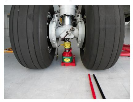
If more than one inch clearance an over the top jack adapter will be required as shown below:
